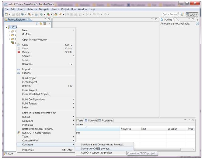
There will be a popup to warn you that some deprecated Add-ins will be removed, equivalent RTE components will not be enabled automatically so you need select them in the system.rteconfig file, refer to ADuCM302x Device Family Pack User's Guide regarding adding RTE configurations. You also need to check the project tool settings to make sure appropriate build settings.
